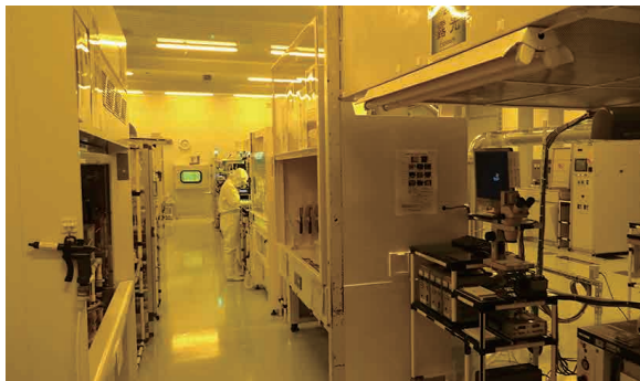
Photo-processing of sensor elements (tuning fork sections) for MEMS gyros. Production is carried out in an area of the cleanroom maintained at the Class 100 standard. Glass discs for rotary encoders are also produced here.
